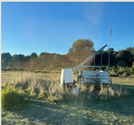
Figure 4: A LIDAR scanner located on site to capture precise wind measurements.
